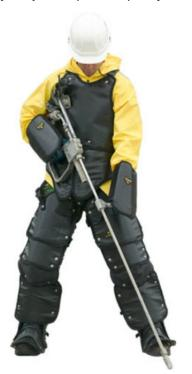
TEST RESULTS: No penetration occured beyond prolective system with waterjet traveling at 2,4 m/s, no closer than 76 mm at these conditions.
